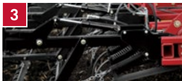
3 Crumbler pressure: achieve consistent clod sizing and finish
